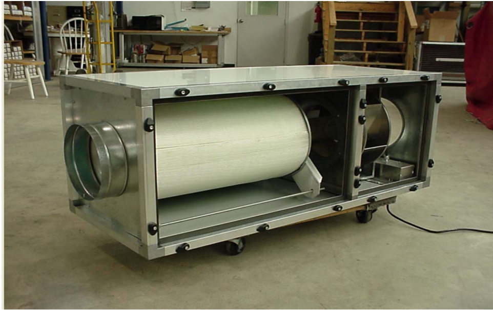
Side view of inexpensive filtration system to make a “Clean Room”. Note: it is in a series with existing HVAC so no major changes need to be made.
